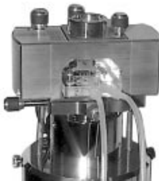
Figure 7.3. Tipholder Inserted into Microscope Head
