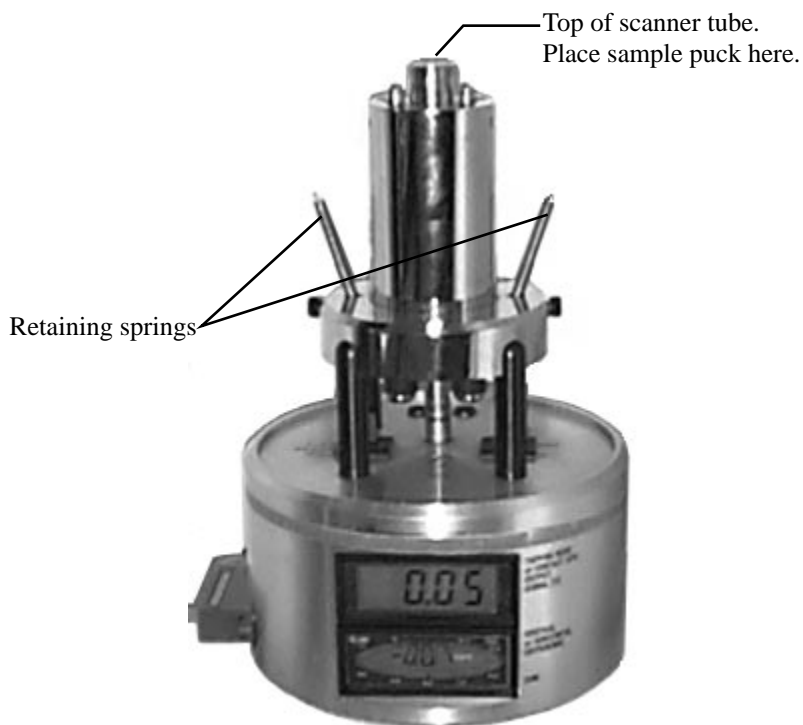
Figure 5.2. MultiMode base with scanner mounted on support ring.
